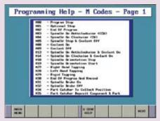
**M-code & G-code** help screens are a quick reference guide when programming at the machine which means you do not have to waste time referring to the manual.
