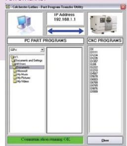
PC front end software for high speed Part Programme transfer over ETHERNET
