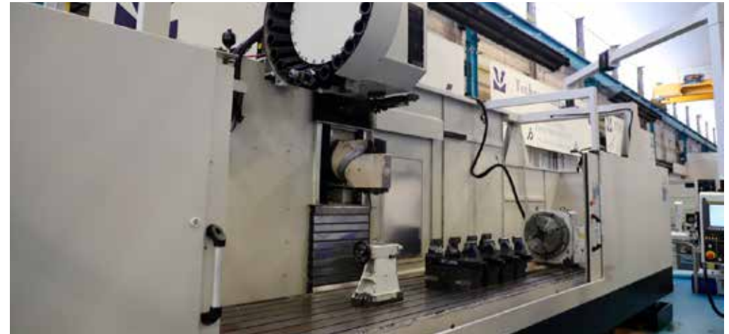
LOT 29: EUMACH FBE 4500 Vertical Machining Centre with Fanuc 31i-Model B control. Table size 4,800mm x 1,050mm. X/Y/Z travels 4,000mm/990mm/1,300mm. 4th axis attachment 500mm dia. Year 2013. Reference CM14
