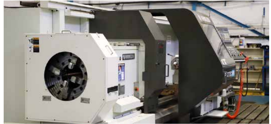
LOT 10: HANKOOK PROTEC 9NC CNC Lathe. Swing over bed 950mm. Swing over saddle 620mm. Distance between centres 4,000mm. Spindle bore 250mm. Fanuc 21i TB Control. Year 2007. Reference CL3
