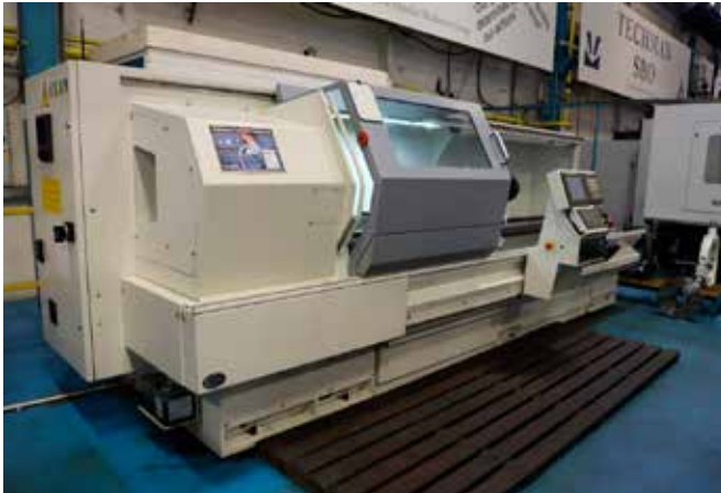
LOT 20: HARRISON Alpha 1550XS CNC Lathe with FANUC 0i-TD Control. Swing over bed 550mm. Swing over saddle 370mm. Distance between centres 3,000mm. Year of Manufacture 2014. Reference CL19
