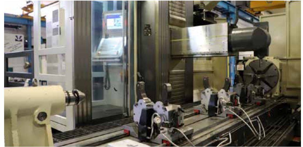
LOT 2: CORREA AXIA CNC Bed Milling Machine with HEIDENHAIN TNC 530i Control Table size 9,000mm x 1,000mm. X/Y/Z Travels 8,500mm/1,500mm/1,250mm 4th Axis attachment 800mm dia. Year of Manufacture 2013. Reference CM18
