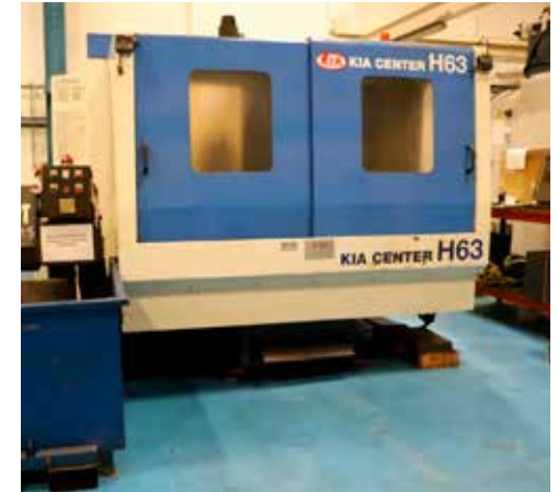
LOT 31: KIA H63 Twin Pallet Horizontal Machining Centre. Pallet size 630mm x 630mm. X/Y/Z travels 950mm/825mm/760mm. B axis. Year 2001. Reference CM20
