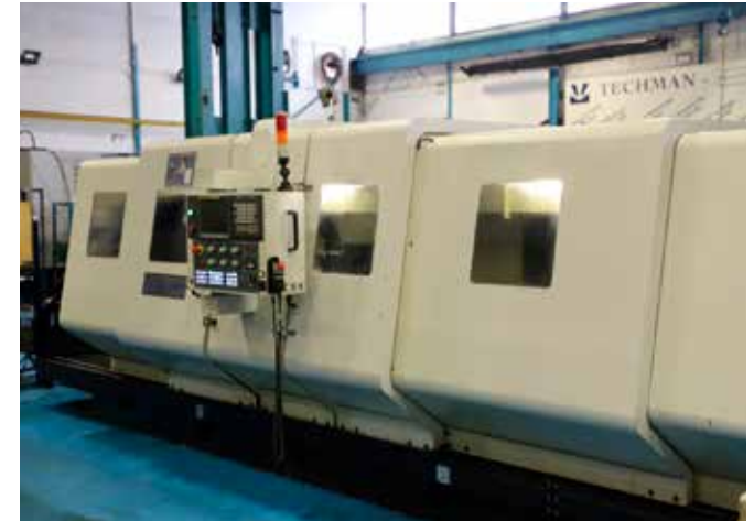
LOT 12: L&L LC38 CNC Lathe. Swing over bed 960mm. Swing over saddle 480mm. Distance between centres 4,000mm. Spindle bore 230mm. FANUC Oi-TD Control. Year of Manufacture 2012. Reference CL16
