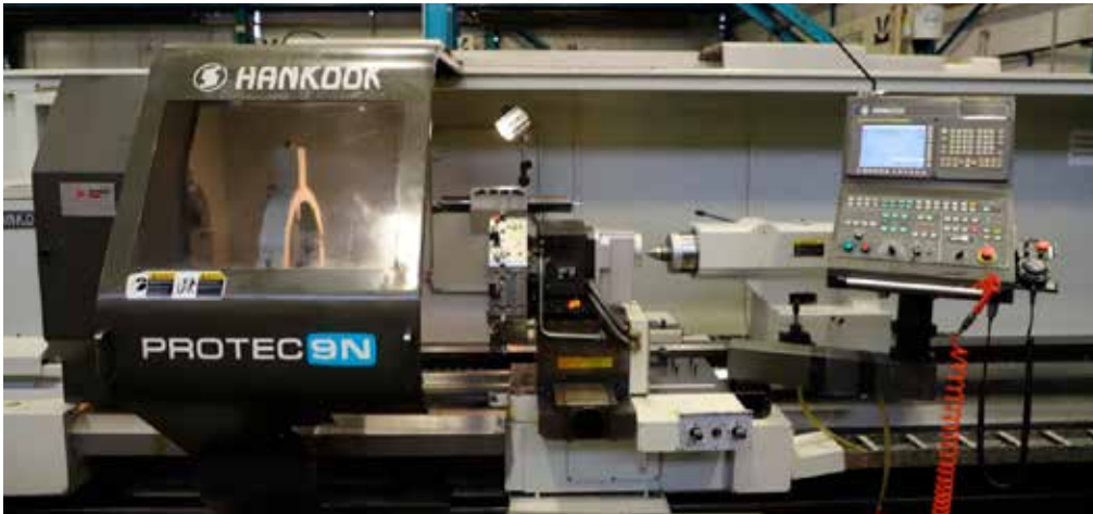
LOT 11: HANKOOK PROTEC 9NC CNC Lathe. Swing over bed 950mm. Swing over saddle 620mm. Distance between centres 4,000mm. Spindle bore 250mm. Fanuc 32i TB Control. Year 2012. Reference CL11
