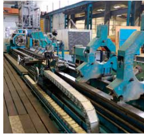
LOT 23: BINNS & BERRY Trident Centre Lathe. Swing over bed 800mm. Swing over saddle 620mm. Distance between centres 12,000mm. Rebuilt in 2008. Reference ML10
