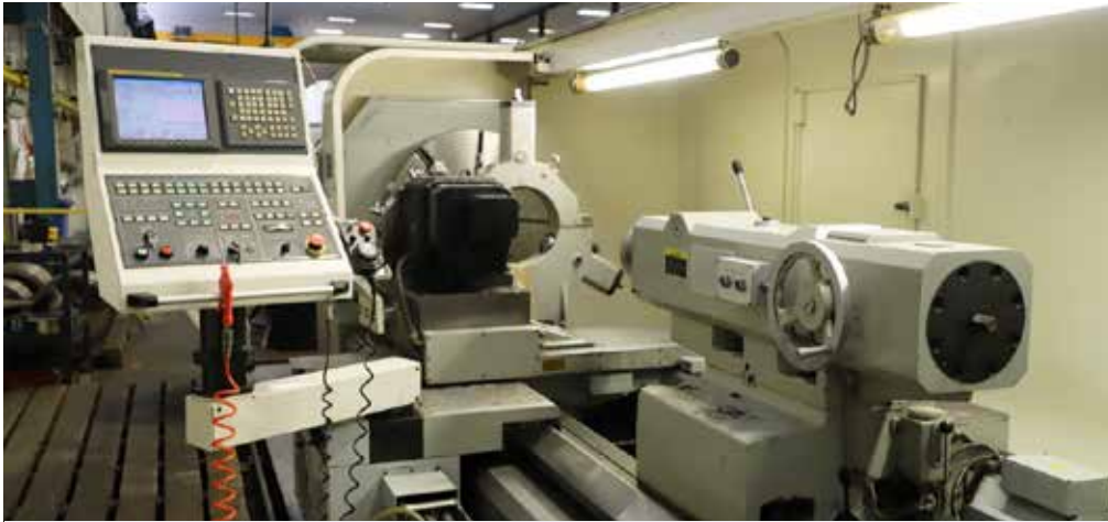
LOT 9: HANKOOK PROTEC 11ND CNC Lathe. Swing over bed 1100mm. Swing over saddle 740mm. Distance between centres 5,000mm. Spindle bore 325mm. Fanuc 21i TB Control. Year 2007. Reference CL4
