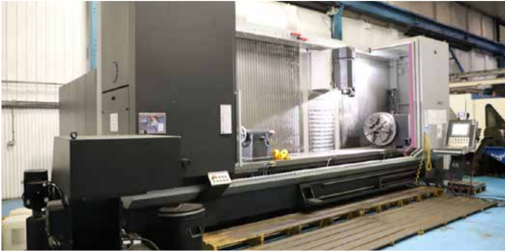
LOT 5: IBARMIA Extreme ZVH4000 CNC Bed Milling Machine with Fanuc 31i Model B control. Table size 5,600mm x 850mm. X/Y/Z travels 4,000mm/800mm/1,050mm. 4th axis attachment 630mm dia. Year of Manufacture 2014. Reference CM17
