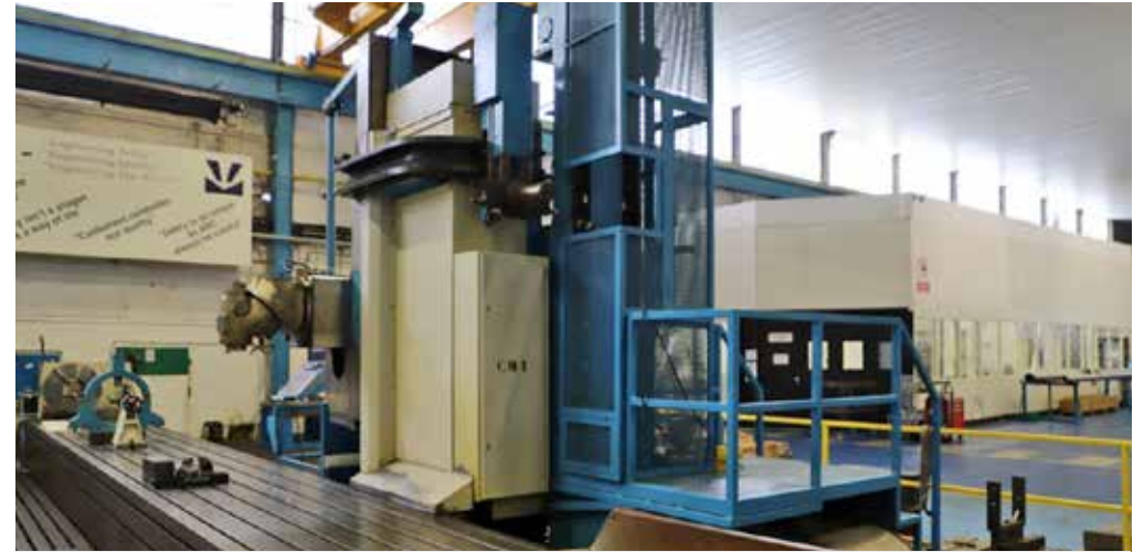
LOT 6: ASQUITH BUTLER HE4000 CNC Bed Milling Machine with HEIDENHAIN TNC 426 Control Table size 10,000mm x 1,180mm. X/Y/Z Travels 8,050mm/1,625mm/1,200mm 4th Axis attachment 630mm dia. Year of Manufacture 1996. Reference CM1
