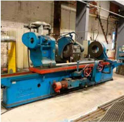
LOT 33: CHURCHILL Cylindrical Grinder. Swing over bed 1,000mm. Thro' spindle tailstock 320mm. Distance between Centres 2,500mm. Reference GR3
