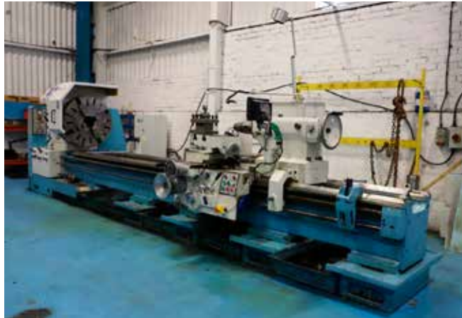
LOT 27: POREBA TPK80 x 4 Centre Lathe. Swing over bed 800mm. Swing over saddle 650mm. Distance between centres 4,000mm. Year of Manufacture 1997. Reference ML6
