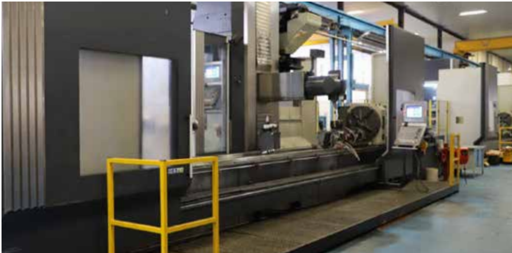
LOT 3: CORREA AXIA CNC Bed Milling Machine with HEIDENHAIN TNC 530i Control Table size 9,000mm x 1,000mm. X/Y/Z Travels 8,500mm/1,500mm/1,250mm 4th Axis attachment 800mm dia. Year of Manufacture 2014. Reference CM19
