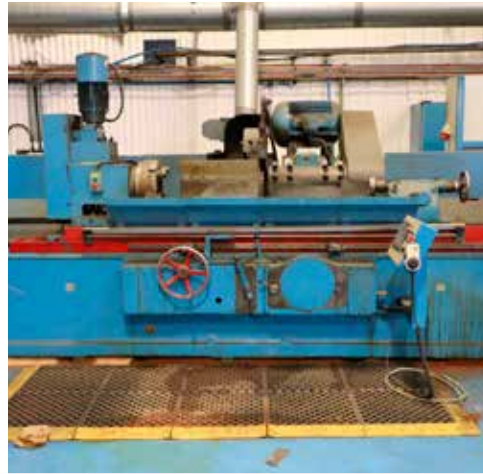
LOT 34: LANDIS MPB CNC Cylindrical Grinder. Swing over bed 500mm. Distance between Centres 1,800mm. Dust extraction unit. Reference GR1
