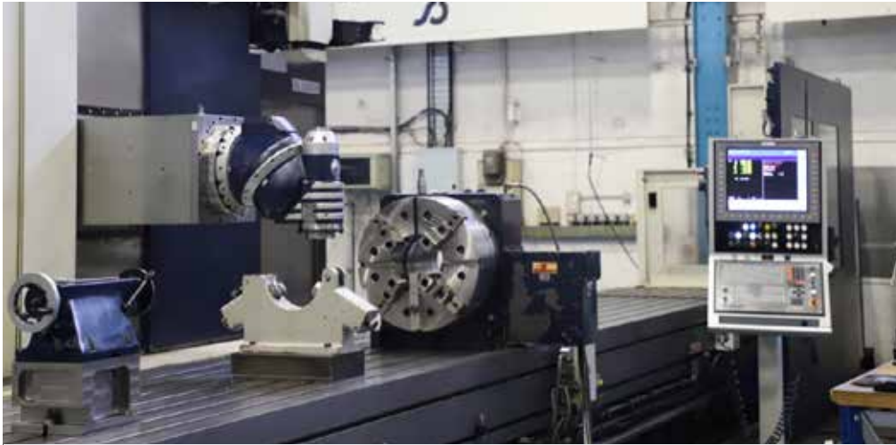
LOT 1: SORALUCE Model SL10000 CNC Bed Milling Machine with HEIDENHAIN TNC530i Control Table size 10,000mm x 1,100mm. X/Y/Z Travels 8,500mm/1,600mm/1,300mm 4th Axis Attachment 630mm dia. x 2. Year of Manufacture 2014. Reference CM16
