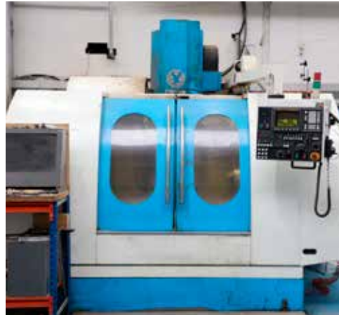
LOT 30: EAGLE Vertical Machining Centre with FANUC O-MD Control. Table size 1,350mm x 550mm. X/Y/Z Travels 1,300mm/600mm/700mm. 4th Axis Attachment 250mm dia. Reference CM4
