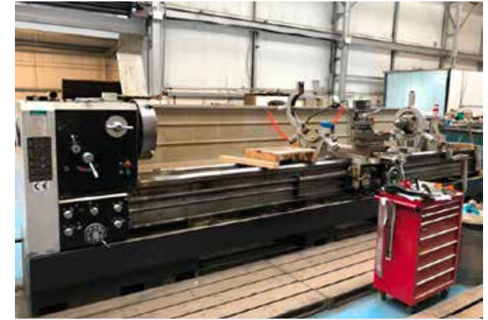
LOT 25: MAS CUT MA-3160 Centre Lathe. Swing over bed 750mm. Swing over saddle 500mm. Distance between centres 4,000mm. Year of Manufacture 2012. Reference ML11
