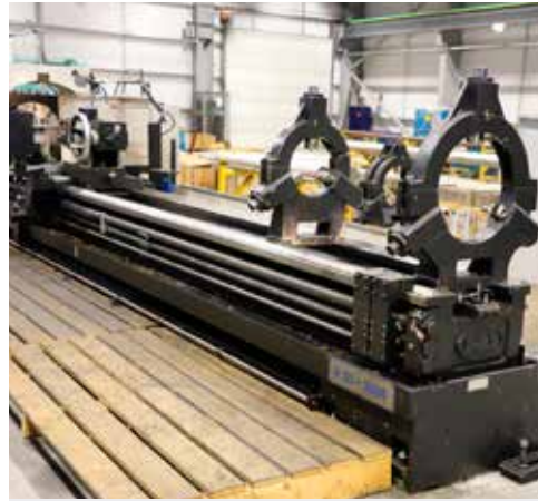
LOT 26: L&L Tuscan A35 x 5000 Centre Lathe. Swing over bed 760mm. Swing over saddle 500mm. Distance between centres 5,000mm. Year of Manufacture 2013. Reference ML14
