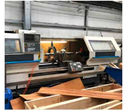
LOT 19: COLCHESTER Mastiff Electronic with FANUC Oi-TD Control. Swing over bed 550mm. Swing over saddle 370mm. Distance between centres 1,800mm. Year of Manufacture 1995. Reference CL6
