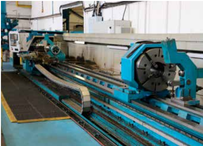
LOT 16: BINNS & BERRY Data 1000 CNC Lathe. Swing over bed 800mm. Swing over saddle 620mm. Distance between centres 12,000mm. FANUC Oi-TC Control. Rebuilt/Retrofitted 2010. Reference CL10
