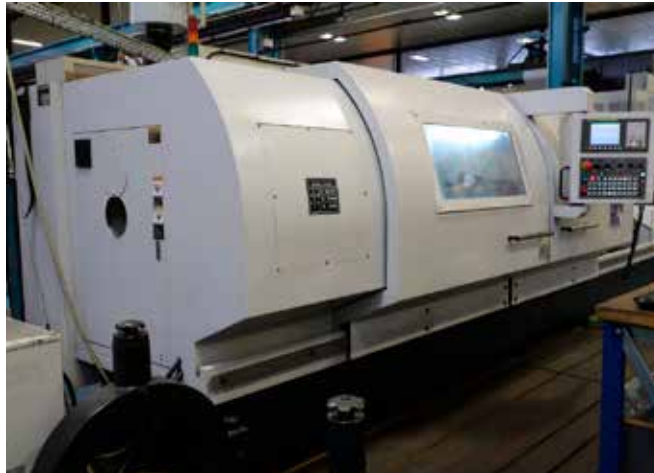
LOT 14: MASCUT AC-25160 CNC Lathe. Swing over bed 670mm. Swing over saddle 400mm. Distance between centres 4,000mm. FANUC Oi-TD Control. Year of Manufacture 2012. Reference CL14
