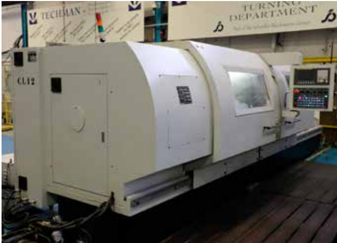
LOT 13: MASCUT AC-25160 CNC Lathe. Swing over bed 670mm. Swing over saddle 400mm. Distance between centres 4,000mm. FANUC Oi-TD Control. Year of Manufacture 2012. Reference CL12
