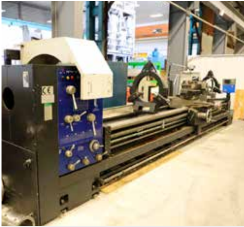
LOT 24: L&L Tuscan A35 x 5000 Centre Lathe. Swing over bed 760mm. Swing over saddle 500mm. Distance between centres 5,000mm. Year of Manufacture 2013. Reference ML12
