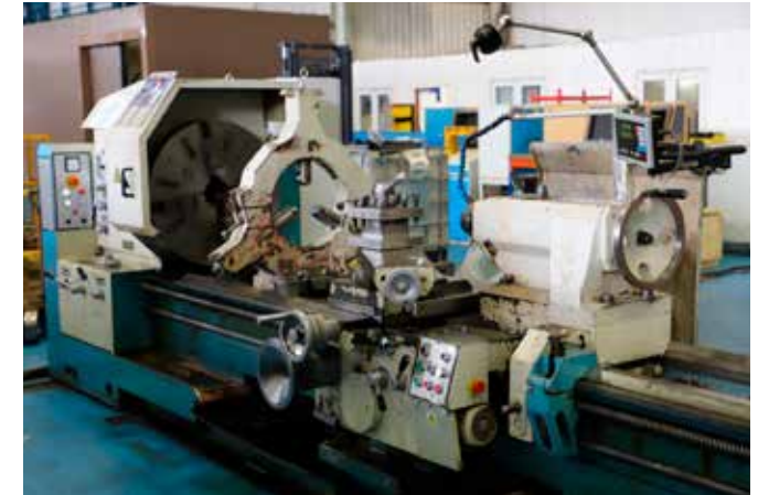
LOT 28: POREBA TPK80 x 5 Centre Lathe. Swing over bed 800mm. Swing over saddle 650mm. Distance between centres 5,000mm. Year of Manufacture 1979. Re-conditioned 2014. Reference ML7
