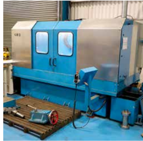
LOT 35: PG MAC CNC Helix Grinding Machine. Swing over bed 485mm. Distance between Centres 1,200mm. Reference GR2
