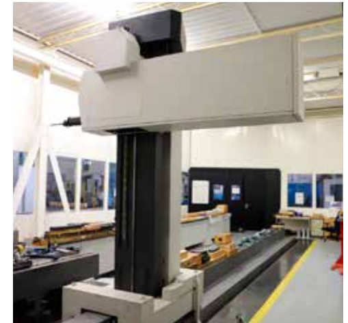
LOT 40: Co-ordinate Measuring Machine Horizontal Arm Type 10,000mm Capacity. Nikken software. Air Conditioning Unit. Tooling/ Probes. Reference INSP1
