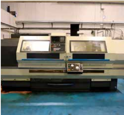
LOT 18: COLCHESTER Mastiff Electronic with FANUC Oi-TD Control. Swing over bed 550mm. Swing over saddle 370mm. Distance between centres 1,800mm. Year of Manufacture 1995. Reference CL7
