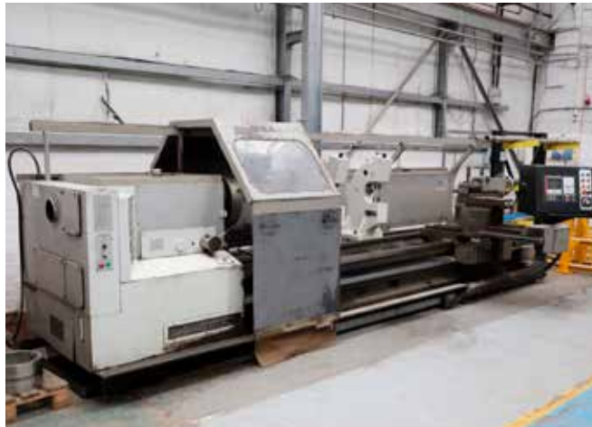
LOT 17: BINNS & BERRY Data 90 CNC Lathe. Swing over bed 900mm. Swing over saddle 720mm. Distance between centres 3,500mm. Retrofitted with FAGOR CNC Control. Retrofitted 1998. Reference CL8
