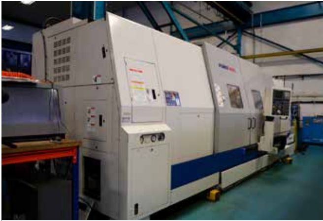
LOT 21: DOOSAN Puma 800L CNC Slant Bed Lathe with FANUC 21i-TB Control. Swing over bed 1,016mm. Maximum Turning dia. 899mm. Maximum turning length 3,200mm. Spindle bore 360mm. Year of Manufacture 2005. Reference CL23
