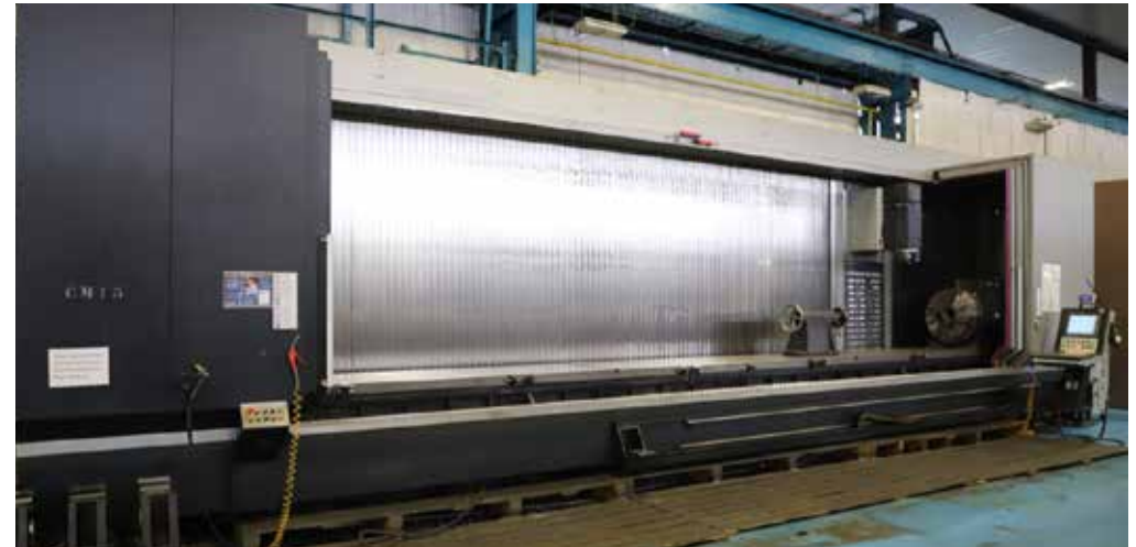
LOT 4: IBARMIA Extreme ZVH8000 CNC Bed Milling Machine with Fanuc 31i Model B control. Table size 9,600mm x 850mm. X/Y/Z travels 8,000mm/1,050mm/1,100mm. 4th axis attachment 630mm dia. Year of Manufacture 2013. Reference CM15
