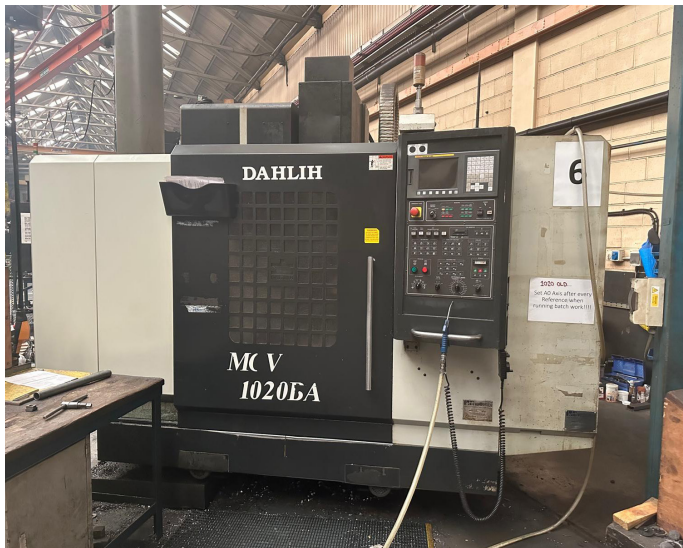
Lot 5: DAHLIH MCV1020BA Vertical Machining Centre with Fanuc Series 0i-MC Control (2007)
