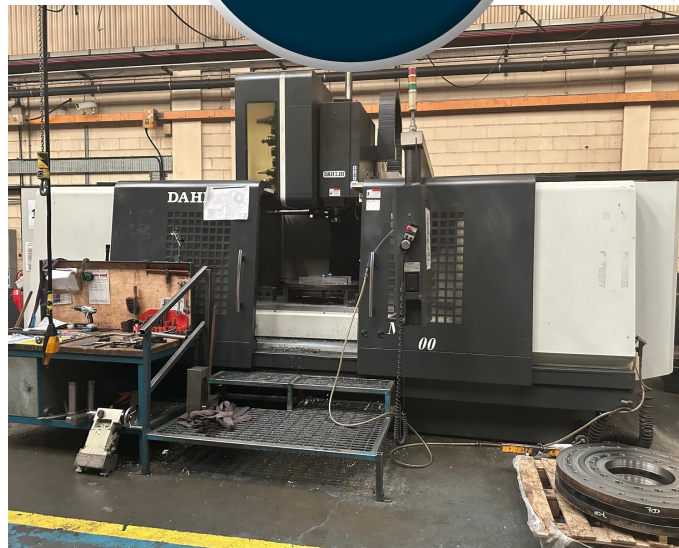
Lot 13: DAHLIH MCV2100 Vertical Machining Centre with Fanuc Series 0i-MD Control (2013)
