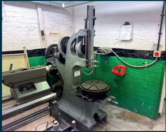
LOT 25. CUNLIFFE & CROOM 6.1/2" Stroke Slotting Machine
