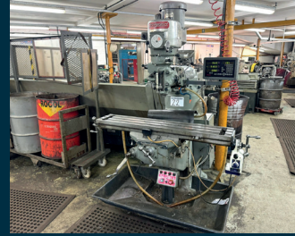
LOT 22. BRIDGEPORT Series 1 Variable Speed Turret Mill with DRO
