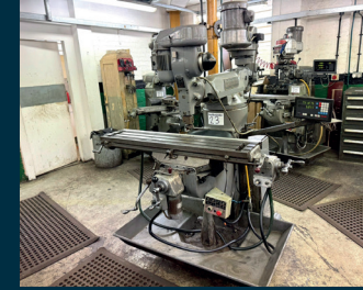
LOT 23. BRIDGEPORT Series 1 2HP Variable Speed Turret Mill with DRO
