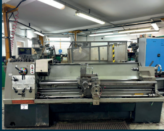
LOT 2. COLCHESTER Mastiff 1400 x 80" Gap Bed Centre Lathe with DRO
