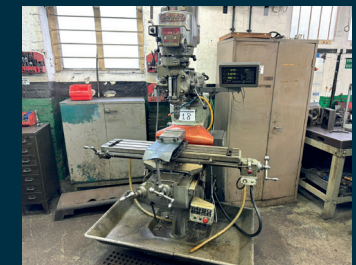
LOT 18. BRIDGEPORT Series 1 2HP Variable Speed Turret Mill with DRO
