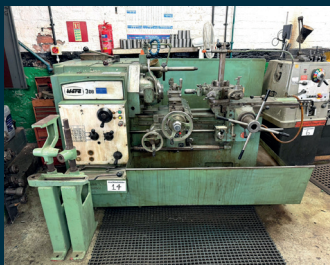
LOT 14. WARD 3DB Capstan Lathe with Collet Chuck and Barfeed
