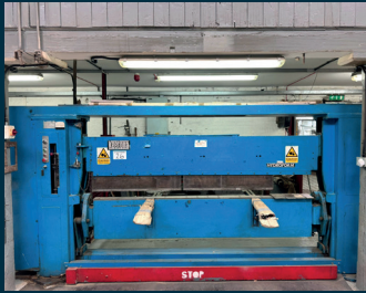
LOT 26. KEETONA Hydroform Hydraulic Folding Machine 100" x 1/8"
