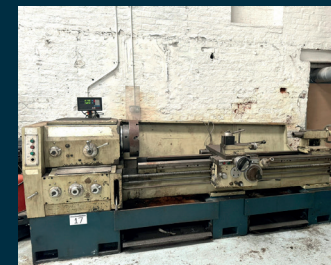
LOT 17. VIKING VT520SB x 78" Gap Bed Centre Lathe DRO
