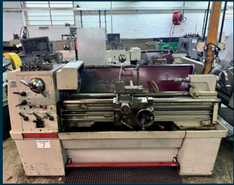
LOT 7. COLCHESTER Triumph 2000 x 50" Gap Bed Centre Lathe with DRO
