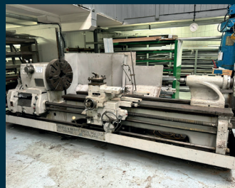
LOT 15. BINNS & BERRY TB x 90" Gap Bed Centre Lathe (Gap Piece Missing)
