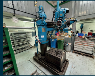
LOT 35. ASQUITH 3'6" Radial Arm Drilling Machine with Box Table
