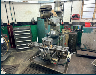
LOT 19. BRIDGEPORT Series 1 2HP Variable Speed Turret Mill with DRO
