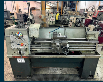
LOT 10. COLCHESTER Master 2500 x 40" Gap Bed Centre Lathe with DRO
