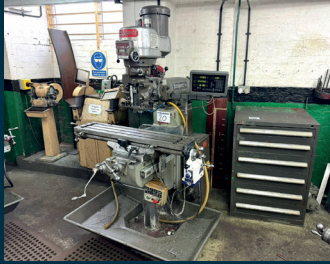
LOT 20. BRIDGEPORT Series 1 2HP Variable Speed Turret Mill with DRO
