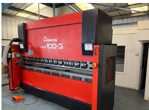
Lot 1: AMADA HFE 100-3 7 Axis CNC Hydraulic Downstroking Pressbrake with SOPE-2 CNC Control. Year 2001
