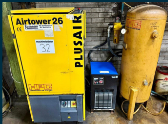
Lot 32: KAESER HPC Air Tower 26 15 Kw Screw Compressor with built in Dryer
