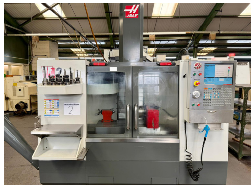
Lot 2: HAAS VF-2 Vertical Machining Centre with 4th Axis Attachment. HAAS Control. Year 2013.
