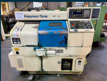
Lot 12: NAKAMURA TOME TMC-15 CNC Lathe with Fanuc Series 18-T Control
