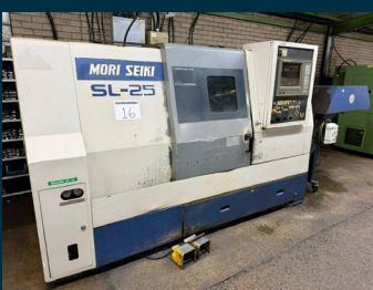
Lot 16: MORI SEIKI SL25B CNC Lathe with Moric-T6FII Fanuc Control
