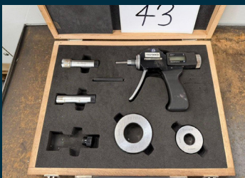
Lot 43: BOWERS XT Holematic 30-35mm Digital Pistol Grip 3 Point Bore Gauge
